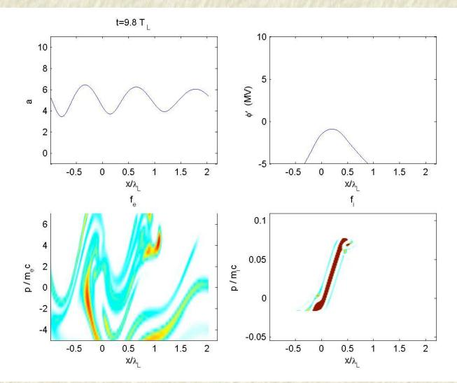
Laser burns through. Poor acceleration.
