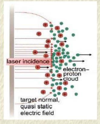
Protons accelerated together with electron cloud as a whole. Could lead to mono-energetic ions in excess of  $100 \,\mathrm{MeV}$ .
