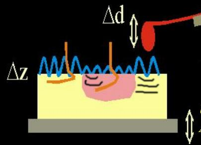
*The cantilever can support highfrequency resonant modes*
