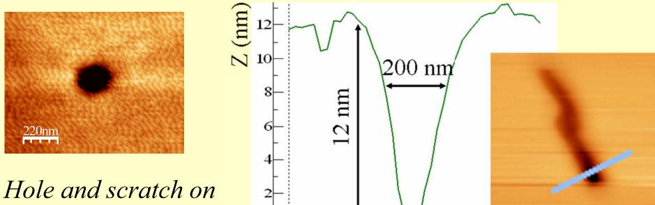
Si(111) by ultrasonic action with an AFM tip
