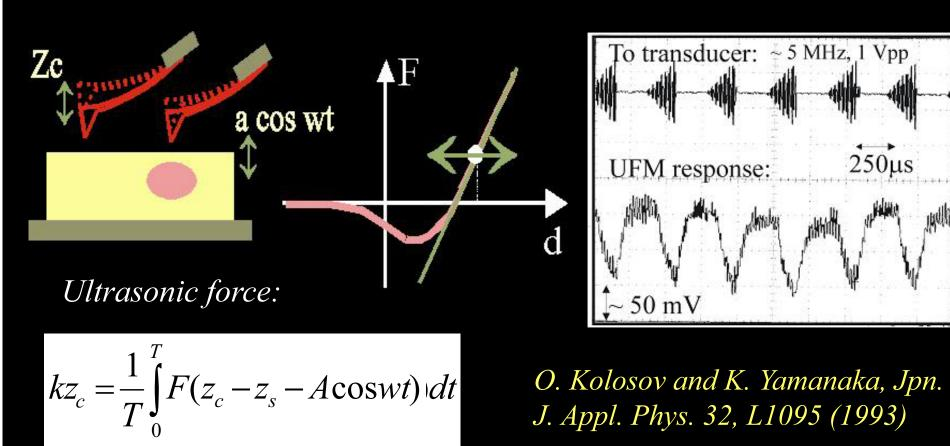
UFM *provides information about* sample elasticity and adhesion with nanoscale lateral resolution. <u>Measured magnitude</u>: static cantilever displacement induced by the *ultrasonic force*.
