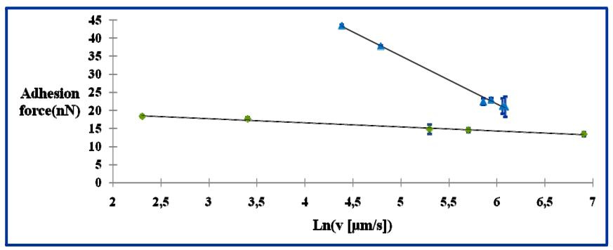
• Intermediate regime for small tip radius (15 nm-green points) and large tip radius (50 nm-blue triangles) at 50% humidity
