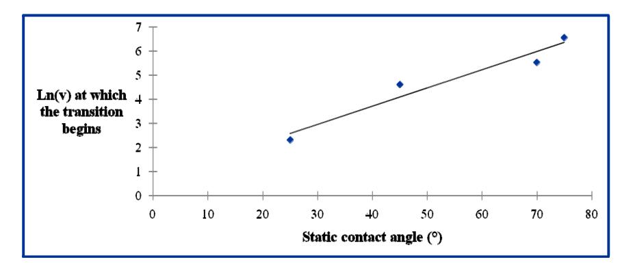
The beginning of the intermediate regime increases linearly with the static contact angle with water Contact angles: *Mica 25°*, *Silicon wafer 45°*, *Silicon nitride 70°*, *Gold 75°*
