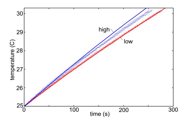
The increase with time of the temperature for surface 2 for two squeezing pressures.
