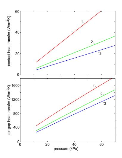
The heat transfer coefficient as a function of the squeezing pressure.
