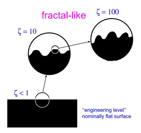
When a nominally flat surface is studied at increasing magnification  $\zeta$ , new surface roughness is detected.
