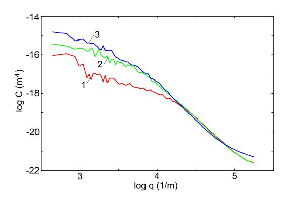
The power spectrum  ${\cal C}(q)$  of the copper surfaces used in the experiment.
