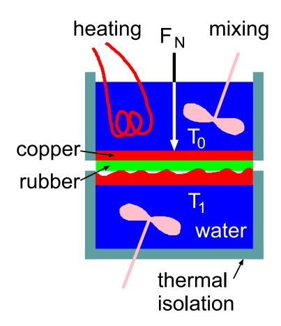
The heat transfer is determined by the temperature increase  $T_1(t)$  in the lower container.
