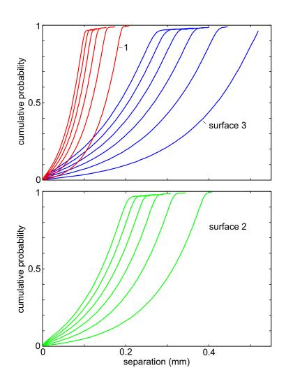
The cumulative height distribution as a function of the interfacial separation for several squeezing pressures.
