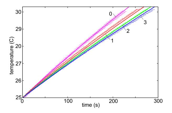
The increase with time of the temperature at fixed squeezing pressure for all 4 surfaces.
