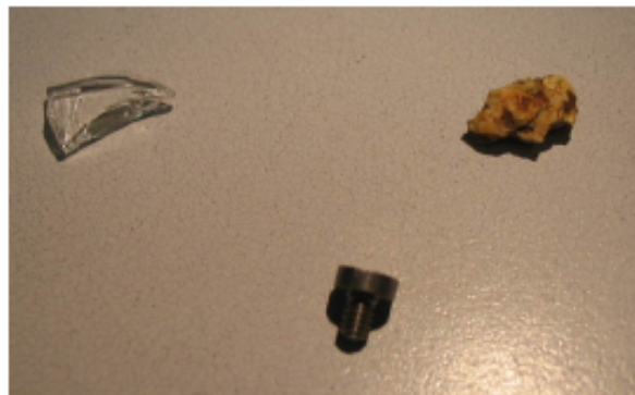
Figure 4. Photograph of different kind of contaminations like a small stone, a glass splinter and a M2 metal screw. The M2 screw may help for size reference.
