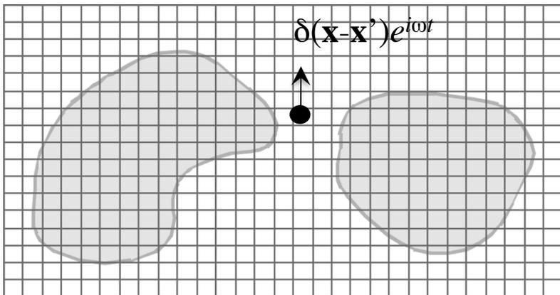
— at every point in space (pixel) and at every frequency  $\omega$ , solve for the Green's function
