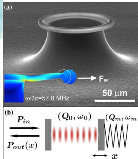
radiation-pressure cooling of microdisk resonators via opto-mechanical coupling
