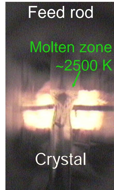
Image furnace grown single crystals now with mean free paths greater than 3000 Å
