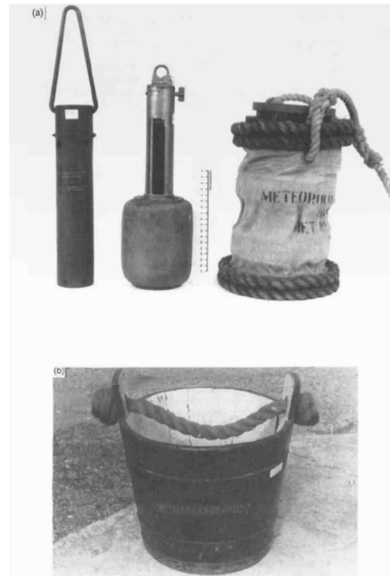
Figure 9. (a) The UK Meteorological Office REF 1800 black insulated bucket, German metal and leather bucket and the UK Meteorological Office Mk II canvas sea temperature bucket and (b) ship's wooden bucket, 1891 (courtesy of Scottish Maritime Museum).
