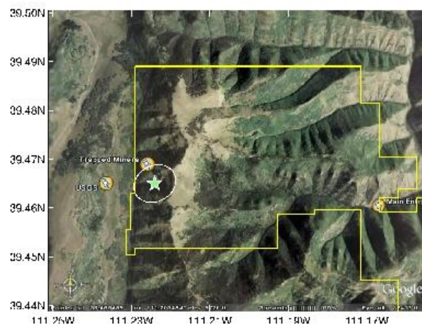
Figure 34: Schema of the Crandall Canyon min and location of mine collapse. Our location of the event (green star) and corresponding 90% confidence ellipse. The left yellow push-pin marks the USGS event location, and the right push-pin is the approximate location of the mine collapse and trapped miners.
