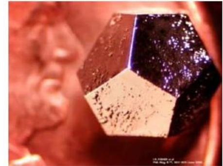
Quasi-crystals = Non-periodic structure with infinite correlations:
