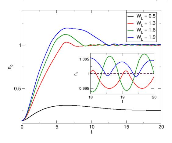
for bias in step region of steady-state picture: no steady state; evolution towards a dynamic state of oscillating density around integer electron number
