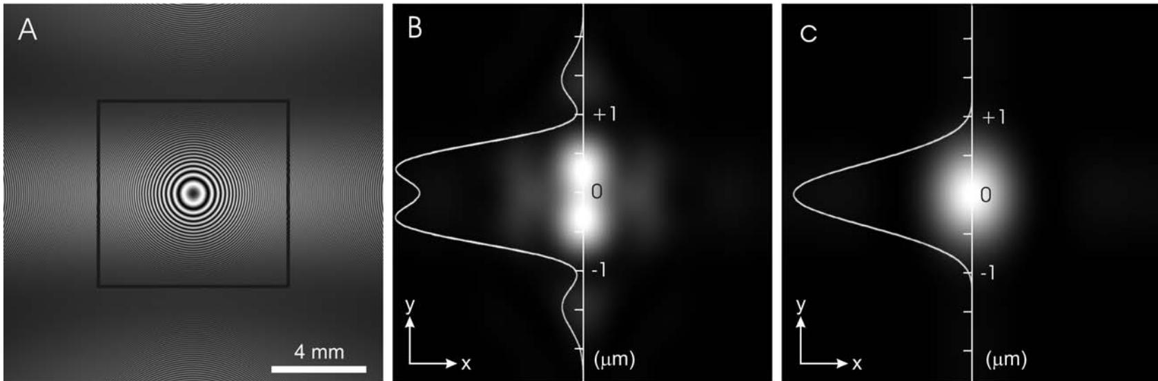
Test of lateral resolution. A: simulated hologram of two points close to the optical axis and 0.8  $\mu\text{m}$  apart, taken with a blue laser  $\lambda=4730\text{\AA}$  with an aperture of 0.5 (0.28 for the inner square). B: reconstruction from the full hologram with the insert showing submicron resolution. C: the same for the smaller hologram losing resolution.
