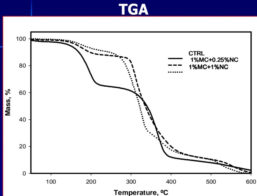
The control sample exhibited two major degradation steps (200 and 370°C).
