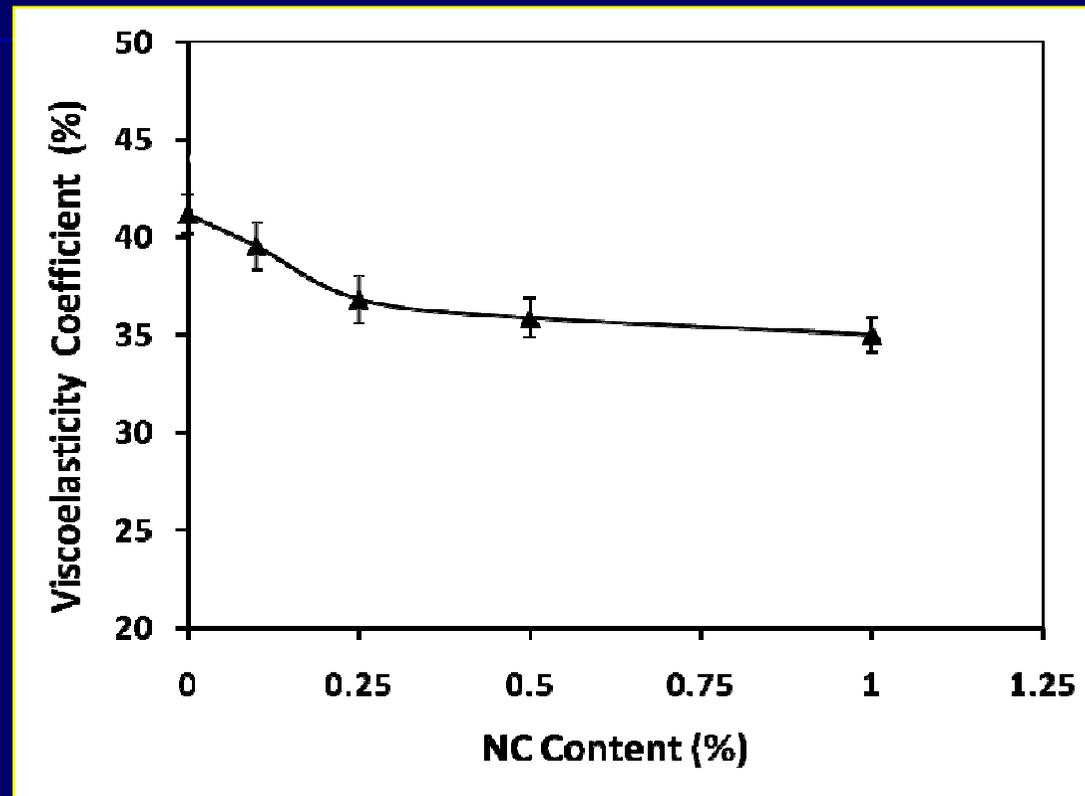
**A monotonous decrease of viscoelasticity coefficient was observed with an increase of NC concentrations in MC-based formulation.**
