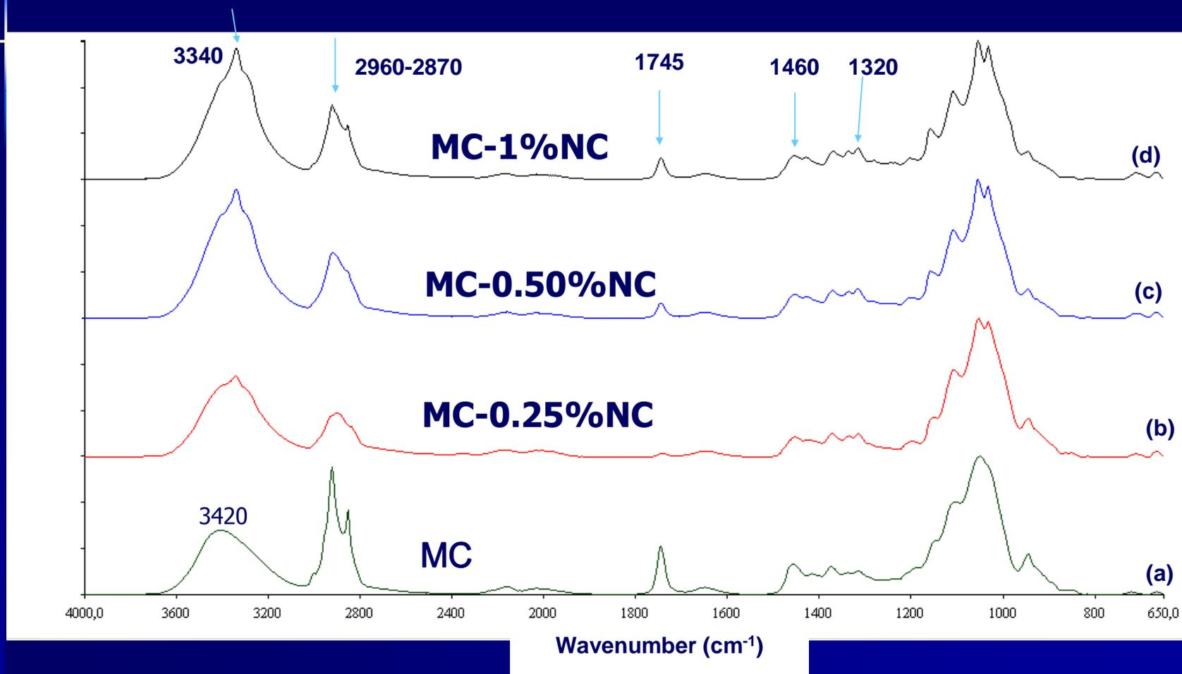
**FTIR spectra of MC- (a) and (MC+NC)-based films containing 0.25% (b), 0.5% (c), and 1% NC (d) respectively.**
