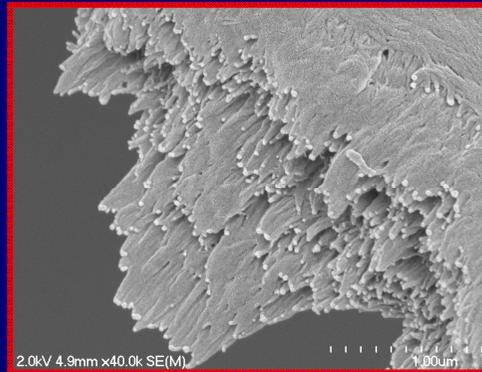
Diameters varied: 2-20 nm, and lengths ranging from a few hundred nanometers up to a few micrometers.
