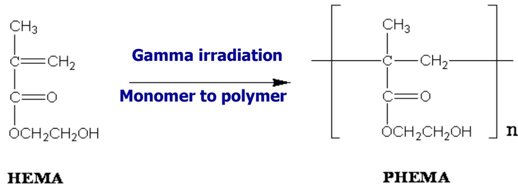
HEMA Monomer is converted to Poly (HEMA) when exposed to gamma Radiation
