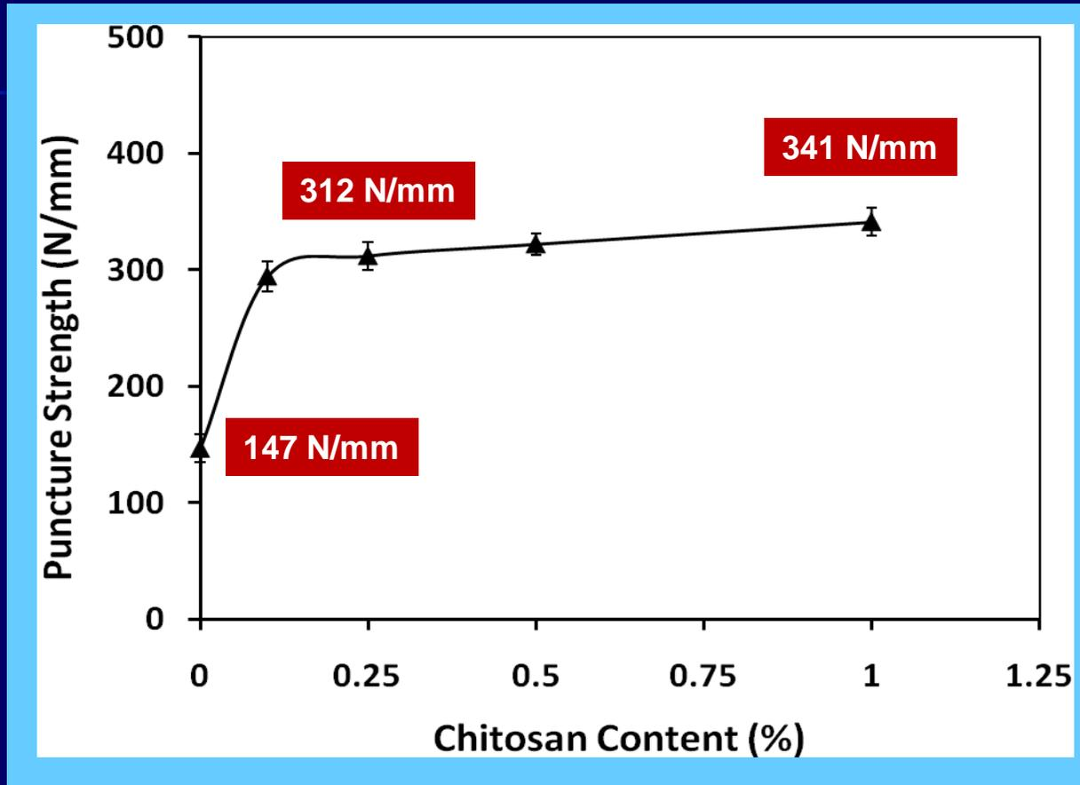
PS of the Chitosan containing films reached to 294, 312, 322, and 341 N/mm, respectively for the addition of 0.1, 0.25, 0.5 and 1% Chitosan solution. It was found that using 0.25% Chitosan solution, the PS improved 117%.
