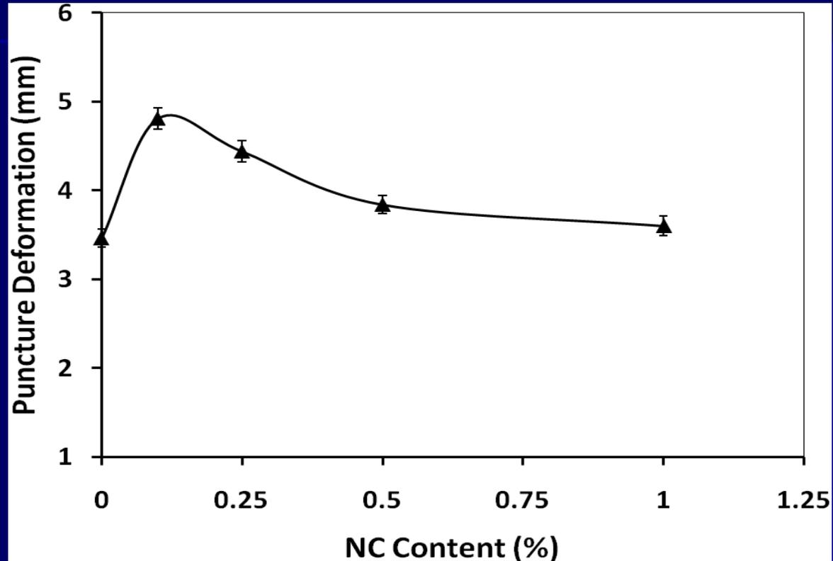
The incorporation of NC caused a significant rise of PD ( $p \leq 0.05$ ). The largest deformation was 39% higher than control, which was observed for 0.1% NC concentration.
