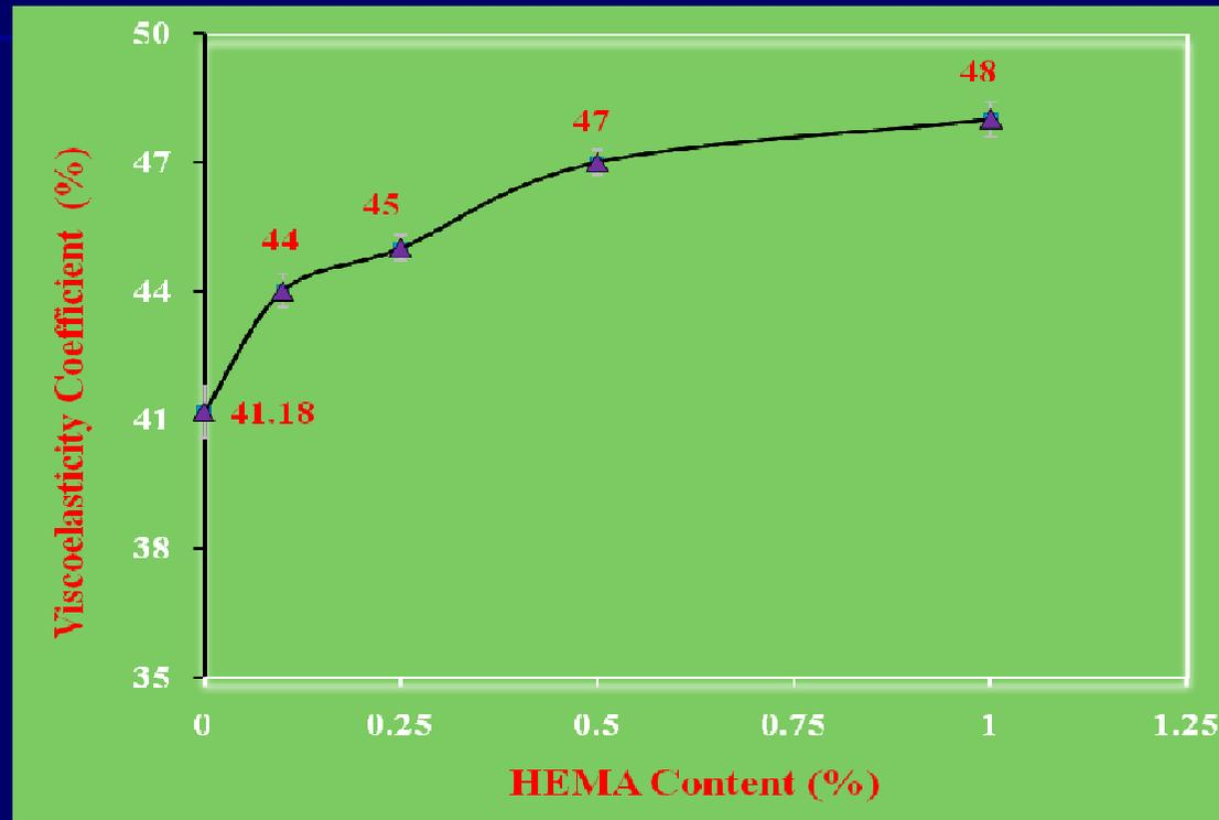
The values of viscoelasticity coefficient of the films also improved significantly when MC-based films were grafted with HEMA monomer at 10 kGy dose.
