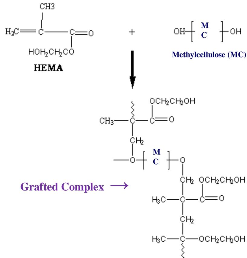
**HEMA monomer reacted with OH groups of methylcellulose in presence of gamma radiation and thus formed grafted complex.**
