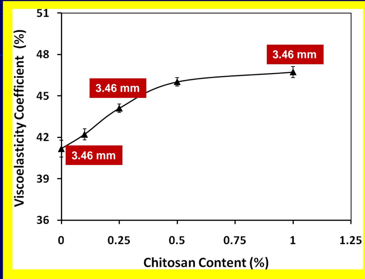
It was found that with the increase of chitosan concentration in the MC-based films, viscoelasticity coefficient values increased linearly.
