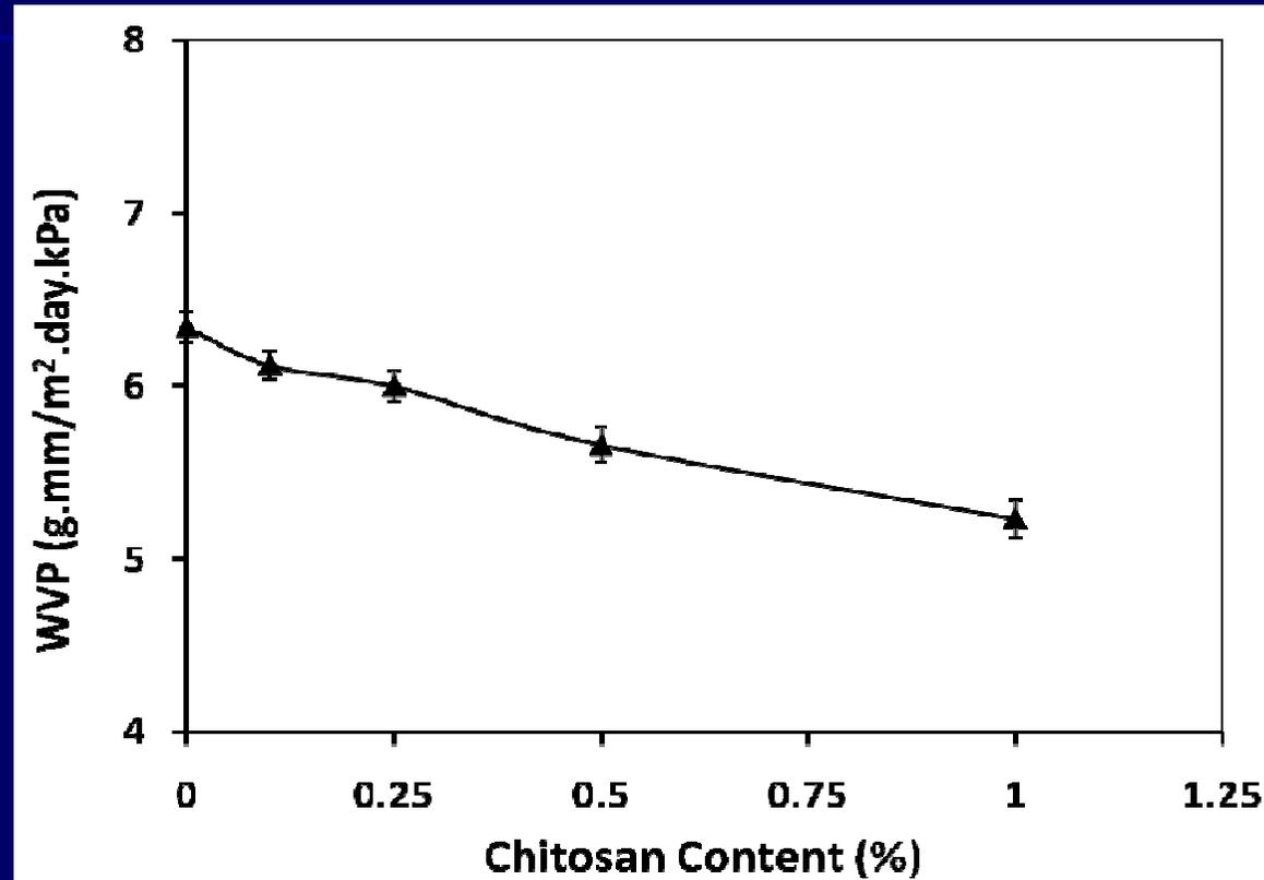
**A 26% reduction of WVP was obtained at 1% Chitosan solution incorporation in MC-based films**
