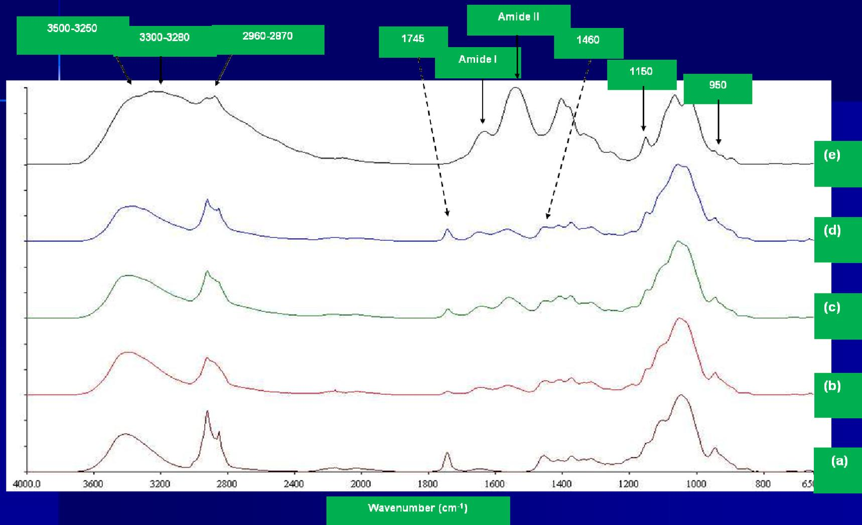
FTIR spectra of MC (a) Chitosan (b) (MC+Chitosan)-based films containing 0.25% (c), 0.5% (d), and 1% Chitosan (e) respectively.
