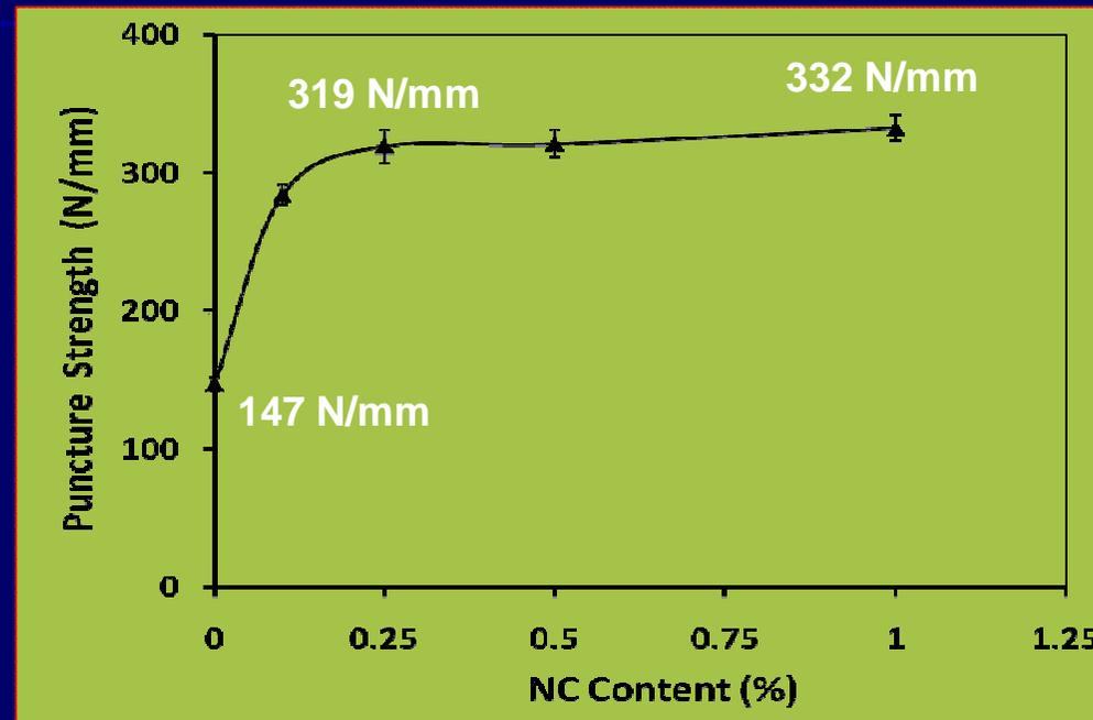
PS of the films reached to 284, 319, 321, 332 N/mm, respectively for the incorporation of 0.1, 0.25, 0.5 and 1% NC solution. It was found that using 0.25% NC solution, PS improved 117%.
