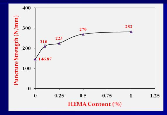
The PS of the films improved significantly (92% improvement for 1% HEMA) when MC-based films were grafted with HEMA monomer at 10 kGy dose. HEMA was successfully grafted with MC by gamma radiation.
