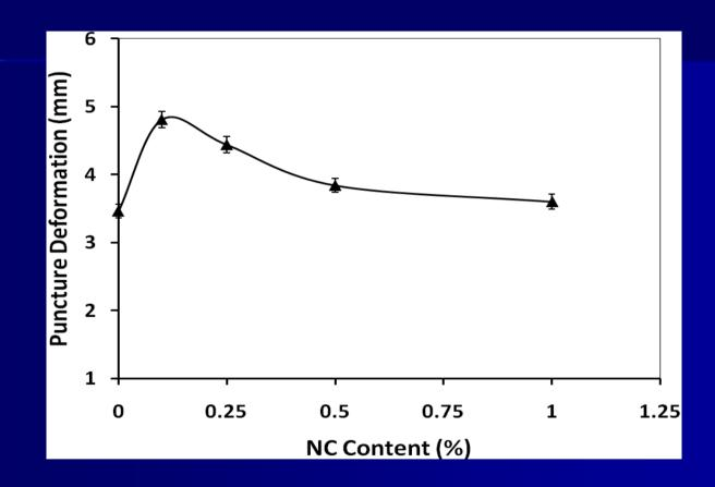
The incorporation of NC caused a significant rise of PD ( $p \le 0.05$ ). The largest deformation was 39% higher than control, which was observed for 0.1% NC concentration.
