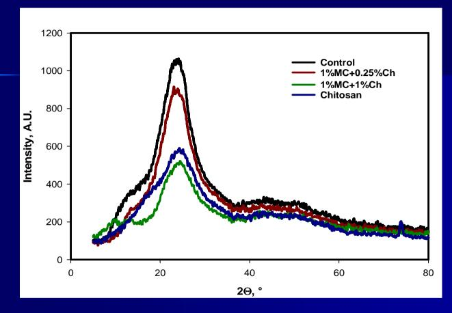
X-Ray Diffractograms for MC- and MC + Chitosan-based films.
