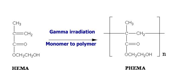
HEMA Monomer is converted to Poly (HEMA) when exposed to gamma Radiation
