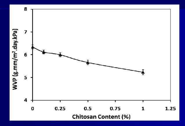
A 26% reduction of WVP was obtained at 1% Chitosan solution incorporation in MC-based films
