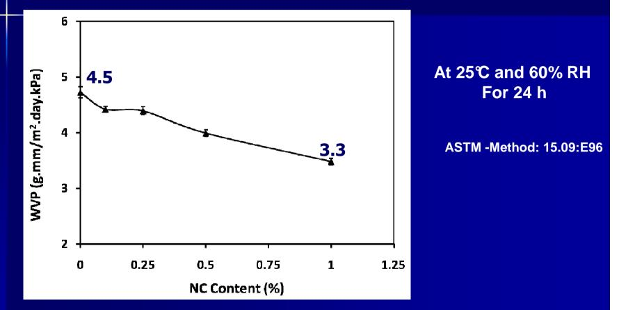
A 26% reduction of WVP was obtained at 1% NC solution incorporation in MC-based films
