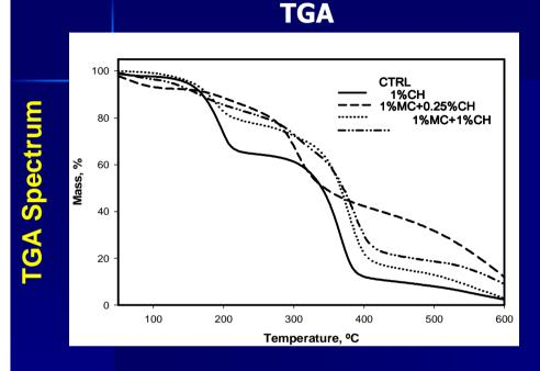
The control sample exhibited two major degradation steps (200 and 370℃).First decomposition: Vegetable oil. Second decomposition: Glycerol and MC. But chitosan containing films found slower degradation.
