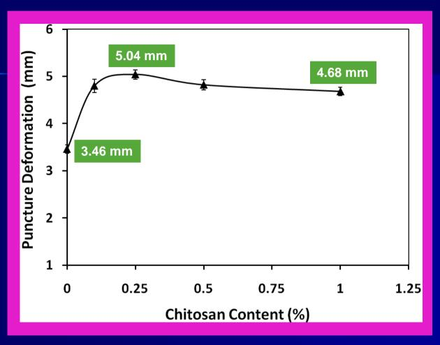
PD values of the Chitosan containing films reached to 4.8, 5.04, 4.82 and 4.68 mm, respectively for the incorporation of 0.1, 0.25, 0.5 and 1% Chitosan solution. It was found that using 0.25% NC solution, PS improved 46%.
