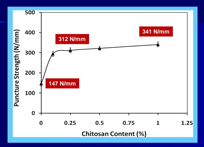
PS of the Chitosan containing films reached to 294, 312, 322, and 341 N/mm, respectively for the addition of 0.1, 0.25, 0.5 and 1% Chitosan solution. It was found that using 0.25% Chitosan solution, the PS improved 117%.
