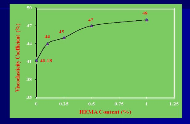
The values of viscoelasticity coefficient of the films also improved significantly when MC-based films were grafted with HEMA monomer at 10 kGy dose.
