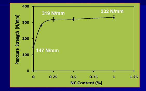
PS of the films reached to 284, 319, 321, 332 N/mm, respectively for the incorporation of 0.1, 0.25, 0.5 and 1% NC solution. It was found that using 0.25% NC solution, PS improved 117%.
