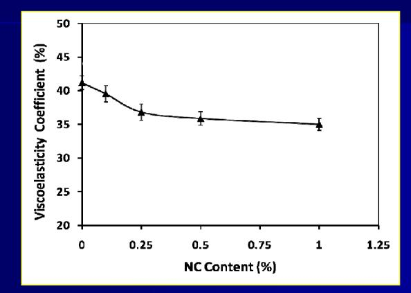
A monotonous decrease of viscoelasticity coefficient was observed with an increase of NC concentrations in MCbased formulation.
