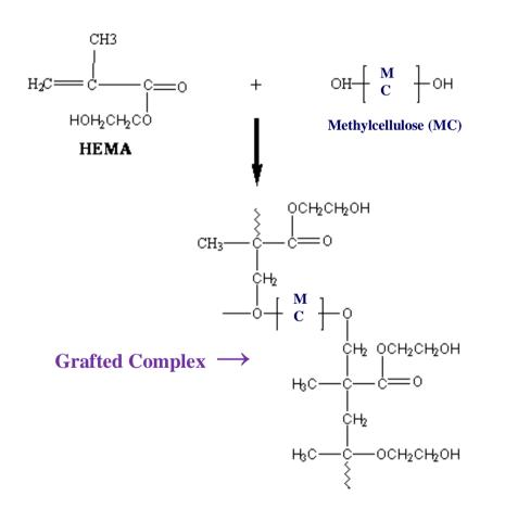
HEMA monomer reacted with OH groups of methylcellulose in presence of gamma radiation and thus formed grafted complex.
