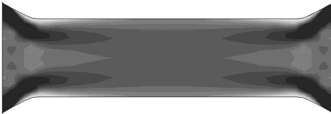
Figure 7.10: Spatial distribution of stress is indicated by levels of shading in a sample with  $r = 2$ , of initial aspect ratio = 3, stretched to  $\lambda = 1.38$ , see Fig. 7.9.
