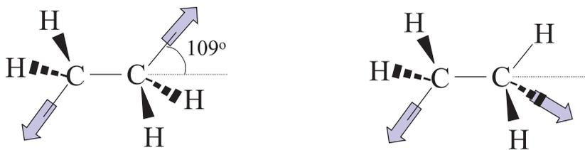
Figure 3.1: The molecular unit (monomer) of a polyethylene chain. Covalent bonds of carbon make a tetrahedron — arrows on the two outgoing bonds show where this unit is connected to other identical monomers, thereby specifying the position of two more C atoms. (a) The *trans* conformation with the  $-\text{C}-\text{C}-$  links in one plane. (b) One of the *gauche* conformations where the first or last C atom is out of plane.
