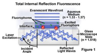
Total internal reflection at the glass/aqueous interface generates an evanescent wave... decays exponentially = illuminates to depth of ~ 100 nm
