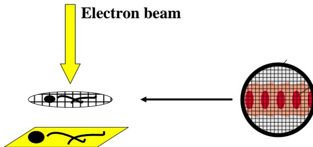
Electrons blocked by objects—resulting « shadows » observed on a phosphorescent screen or captured on photographic film
