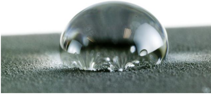
Water drop on a super-hydrophobic surface ( www.itg.uiuc.edu )
