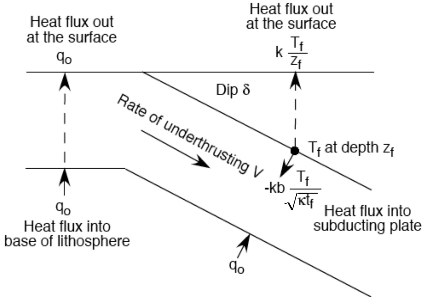
Steady-State temperature in a thrust fault setting: no frictional heating (yet)
