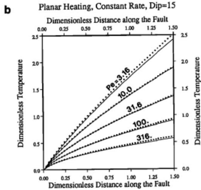
Numerical solutions for temperature along thrust faults
