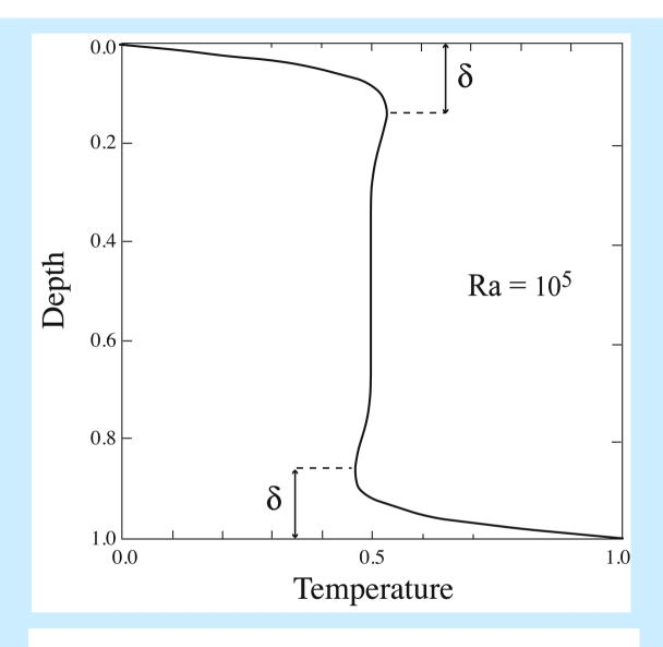
$$\overline{q} = -\lambda \frac{\partial \overline{T}}{\partial z} + \rho C_p \overline{w\theta} = \text{constant} = Q,$$
