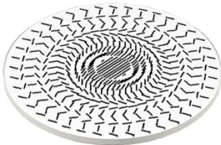
The lens **thickness will be uniform and very thin** (few microns). Similar to Fresnel lens, but without optical discontinuities
