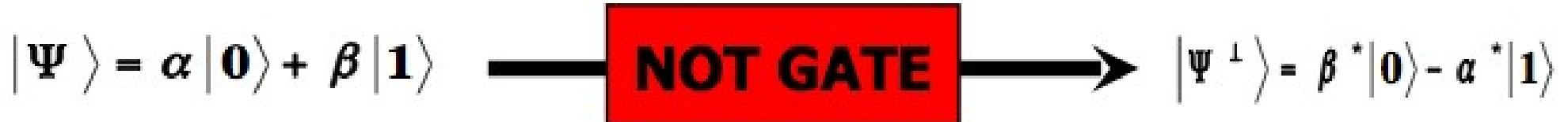
Inversion of the Bloch sphere: Flipping of a qubit on the symmetric point of the Bloch sphere
