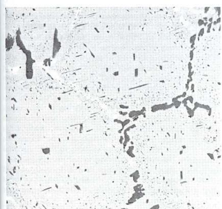
Microstructure of the HP 45 stainless steel after treatment with a low hydrogen pressure of 0.1 Pa for 100 h at 1200 K.
