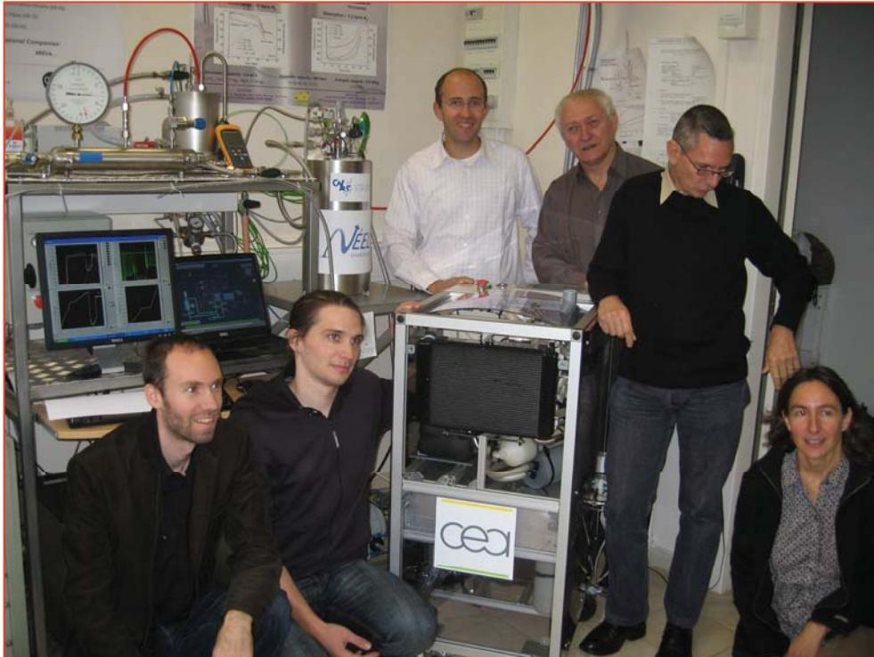
**Connection to the «EPICEA» PEM-FC of CEA, Grenoble (4 kW, effic. ~ 50%, 2 kW electric) here powering for ~ 1 h. a ancillary heater**
