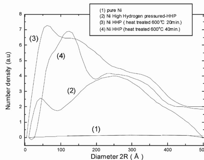
Size distribution of nanopores in Ni submitted to a HHP of 3.5 GPa at 800 °C for 5 h, and subsequently heat treated at 600 °C for 20 and 40 min.
