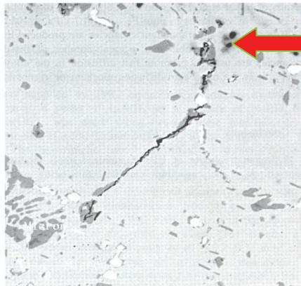
Microstructure of the HP 45 stainless steel after treatment with a high-hydrogen pressure of 5 GPa for 1 h at 873 K.
