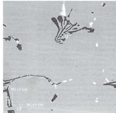
Typical micrograph of the HP 45 stainless steel with Nb and Ti additions in the as-cast condition.
