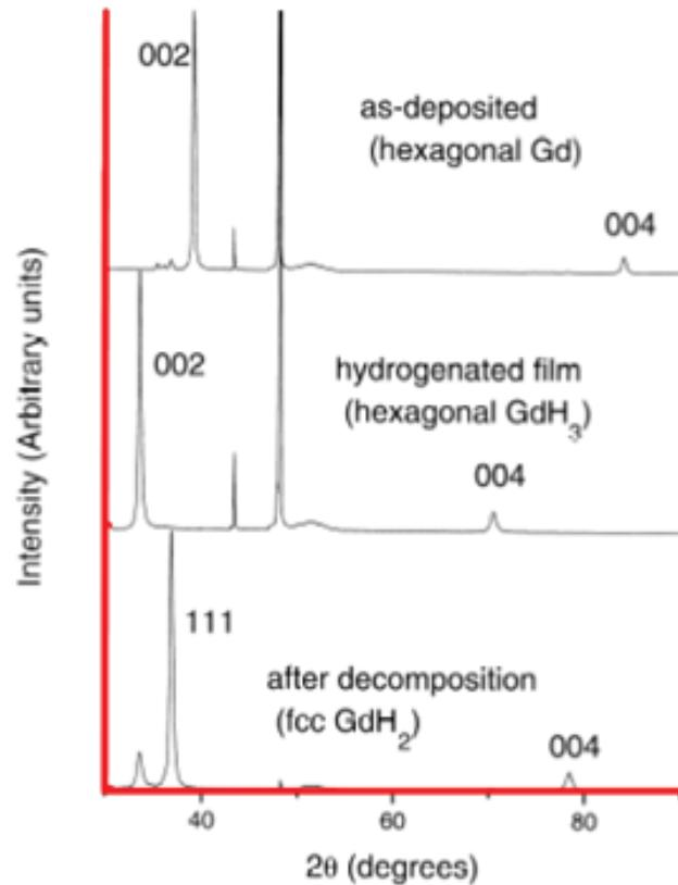
X-ray diffraction patterns of an as-deposited film (top), a hydrogenated film (center) and a film after decomposition (bottom).
