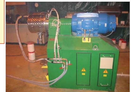
Energetic Ball-Milling is a common method used to prepare reactive powders : homogeneous nano-crystallites, high density of defects, doping with metal type catalysts®
