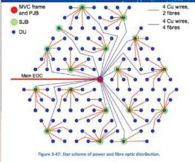
Figure 3-47: Star scheme of power and fibre optic distribution.
