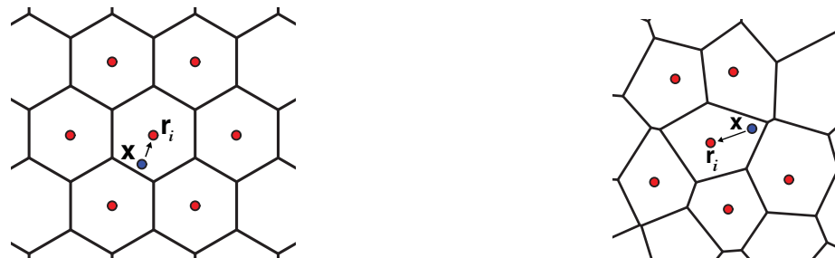
Figure 4: Any point \mathbf{x} is quantized (“rounded-off”) to the nearest point \mathbf{r}_i . Left panel: Triangular lattice. Right panel: Irregular point process.
