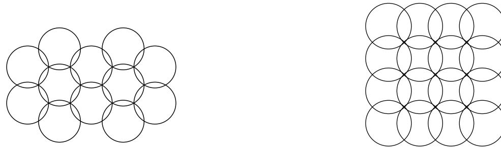
Figure 2: Coverings of the plane with overlapping circles centered on the triangular lattice ( \theta = 2\pi/(3\sqrt{3}) = 1.2092\dots ) and the square lattice ( \theta = \pi/2 = 1.5708\dots ).
