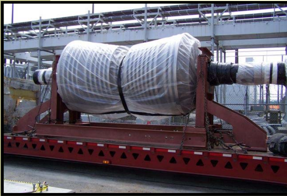
High Pressure Turbine for Unit 2 being delivered
