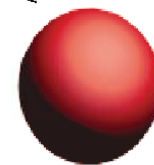
Dia. 0,5mm Uranium Dioxide Fuel Kernel
