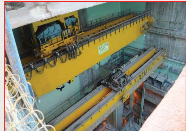
33m girders & trolley of 280/85 T EOT in RCB
