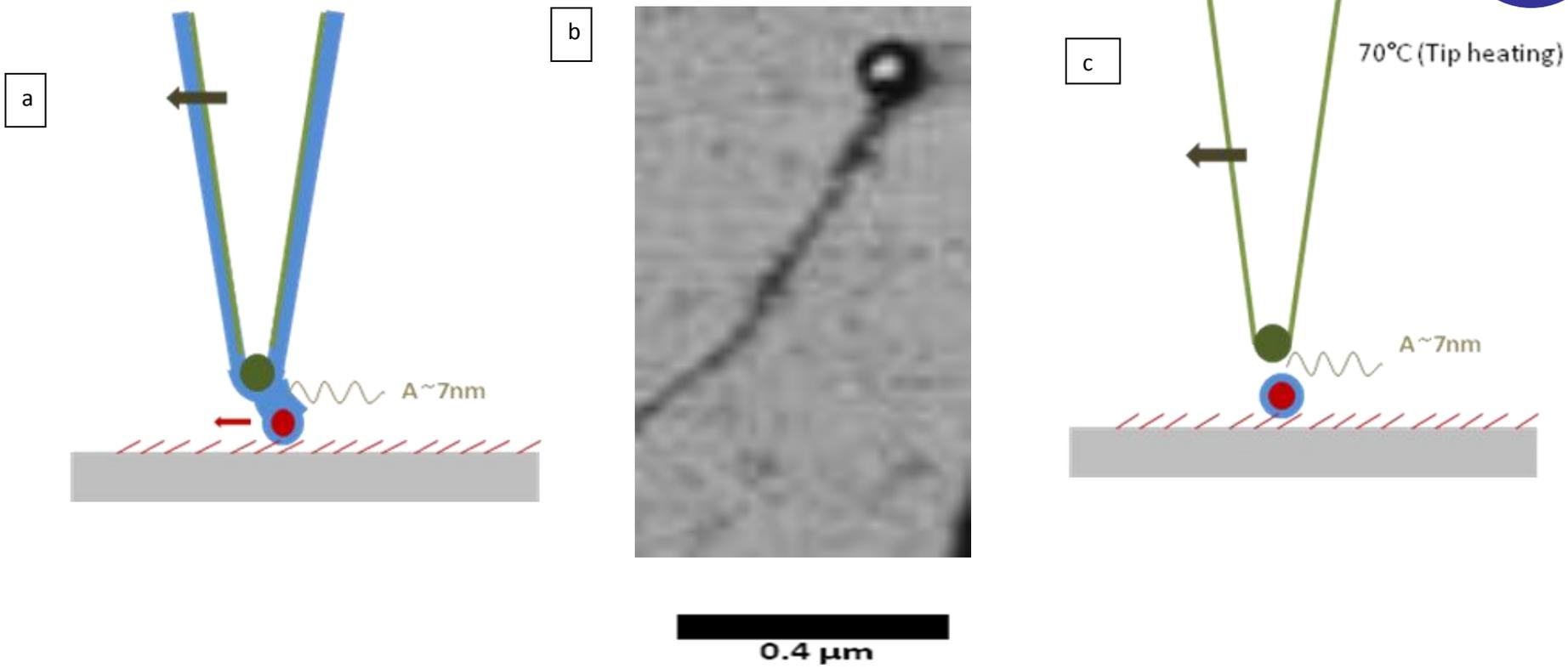
Schemes of the system configuration (hydrophilic particle/ hydrophobic substrate/ partially hydrophilic tip) at 80 % of RH using low  $A_{set}$  and drive amplitude (tapping parameters): a) tip pulling NP via the capillary bridge between the tip/NP and c) fixed NP after heating of the tip. b) AFM phase image in tapping mode, during the manipulation of NP; the black line corresponds to the trajectory of the particle (slow scan axis down).
