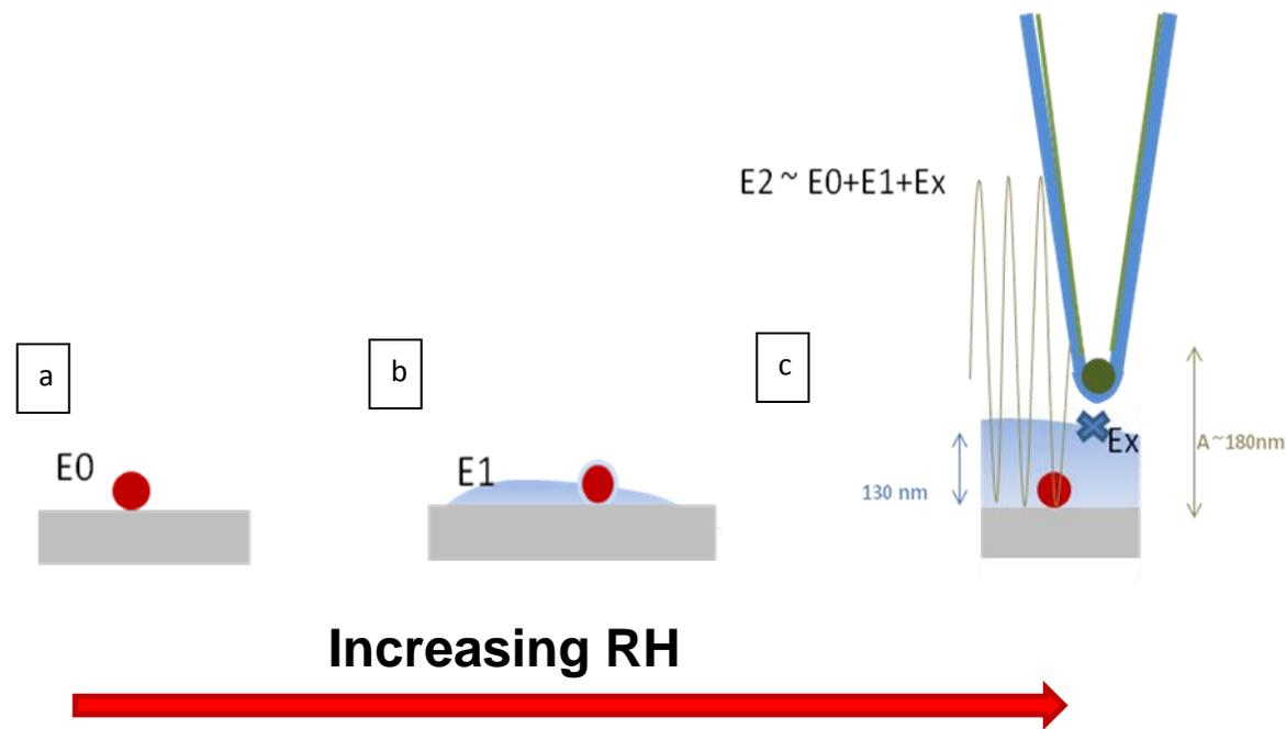
Evolution of the threshold energy dissipation (eV) to move citrate coated NPs (hydrophilic) on SiO<sub>2</sub> (partially hydrophilic) vs the relative humidity. At 2 % of RH the pressure was 10 mbar and it is the reference value to move these NPs on such substrates.
