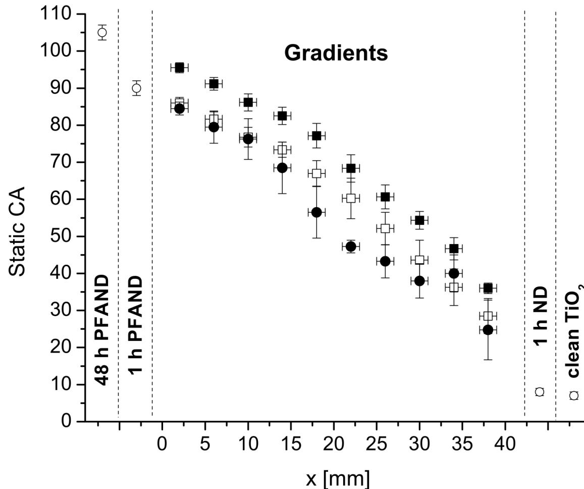
PFAND one-component (■), ND backfilled gradients (□), after their additional immersion in  $\text{H}_2\text{O}$  for 14 h
