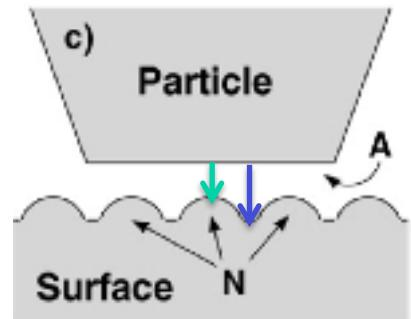
$$F_{\text{adh}} = \frac{A_H A}{6H_0^2} \left[ \rho r + \frac{1}{\pi H_0 (1 + y_{\max}/H_0)^3} \right].$$
