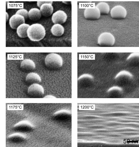
Sintering of particles at different heat-treatment temperatures
