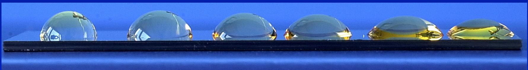
A Simple, Reproducible Approach to the Preparation of Surface-Chemical Gradients
