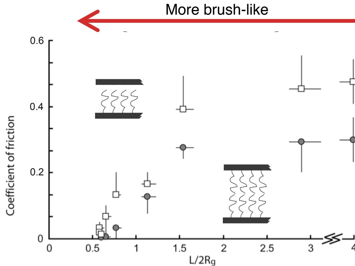
Possible interpretation: at low loads, stiff brushes help separate sliding surfaces and lead to low-friction sliding across solvent-rich interface.
