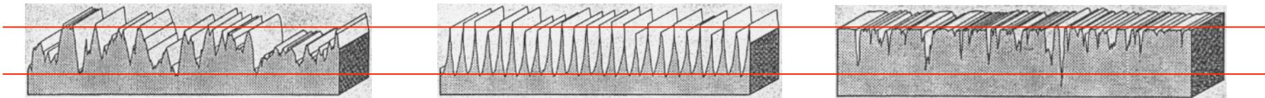
Amplitude Parameters (e.g. Ra) are identical, Spacing and Statistical Parameter are different
