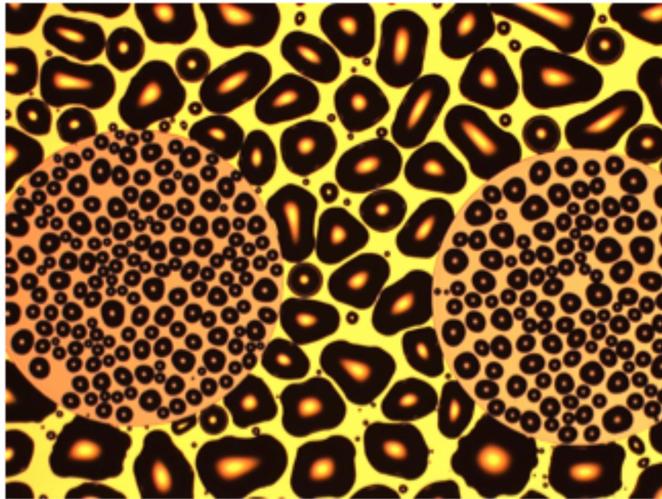
Simultaneous adsorption of OH-terminated thiol and PFAND on an ultraflat Au and Ti surface (microdroplet density image)
