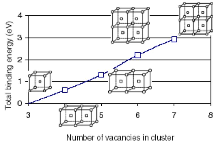
Fig. 2. Total binding energy for vacancy clusters versus the number of vacancies in the void.
