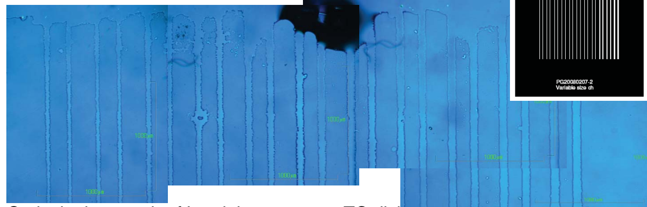
Optical micrograph of Laminin pattern on TC dish
