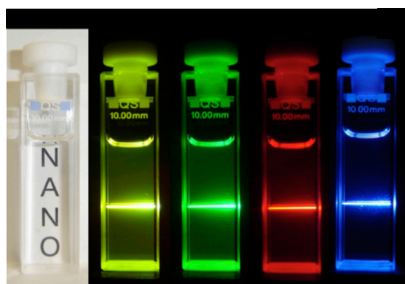
Fig. 1: Digital image of UCNPs doped with various lanthanide ions following 980 nm excitation.
