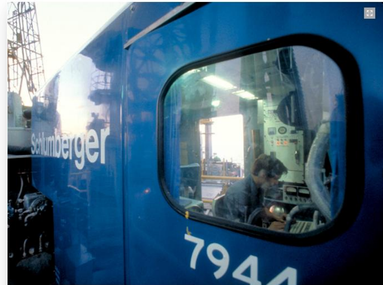
CSU Cabin. Log data could now be transmitted from the field by telephone or satellite. By 1976, the first logging truck equipped with a computer, known as CSU* wellsite surface instrumentation, went into service.
