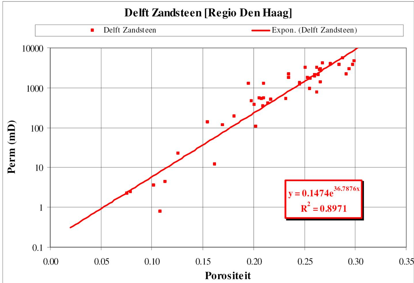
Porosity – permeability relationship from measurements on core in the laboratory
