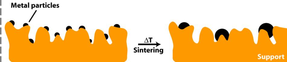
Sintering due to thermal treatments decreases the catalytic activity
