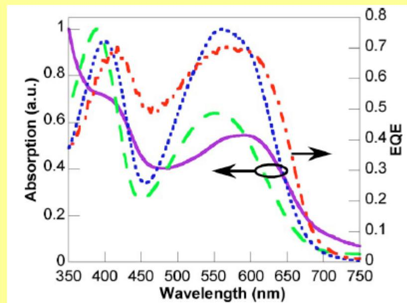
Absorption spectra of PSiF-DBT film (dot), solution (broken) and PSiF-DBT:PC60BM 1:2, w/w blend film (solid) and the EQE of the PSC.
