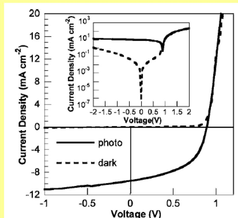
*I-V* curve of the device *ITO/PEDOT:PSS/PSiF-DBT:PC60BM 1:2, w/w/Al, AM 1.5 G 800 Wm<sup>-2</sup>*.
