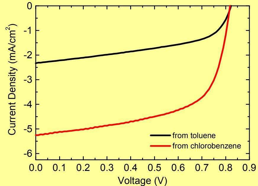
A 2-3 fold increase of the IPCE and short circuit current was observed by S.E. Shaheen et al.\* due to the change from toluene to chlorobenzene as solvent, while by AFM measurements a decrease in the surface roughness was detected.
