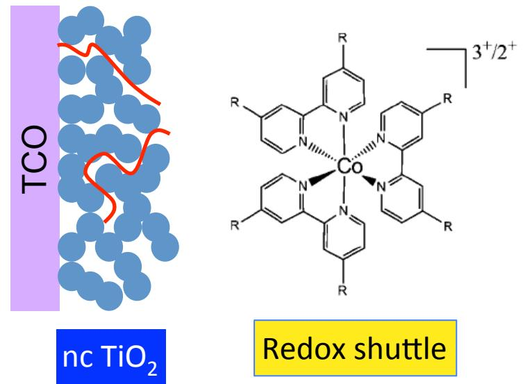
Enlargement of pore size from 23 nm to 32 nm avoids mass transfer limitation of photo current.
