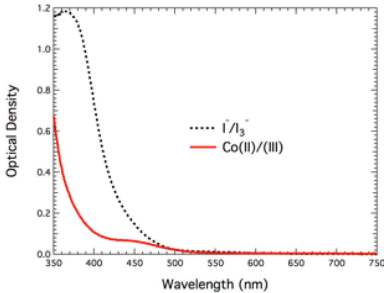
Absorption spectra of  $\text{Co(II)/Co(III)}$  and  $\text{I}^-/\text{I}_3^-$  based electrolytes
