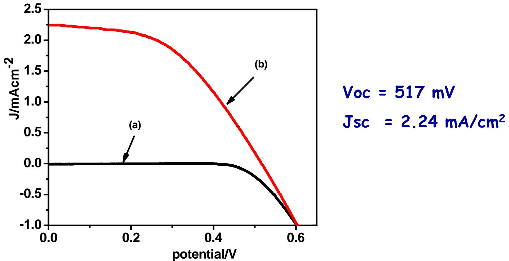
J-V characteristics of ITO/nc-TiO<sub>2</sub>:SH-dye/PVP:CH<sub>3</sub>CN:I<sub>3</sub><sup>-</sup>:EMImI/PEDOT/ITO cell (a) in the dark and (b) under illumination
