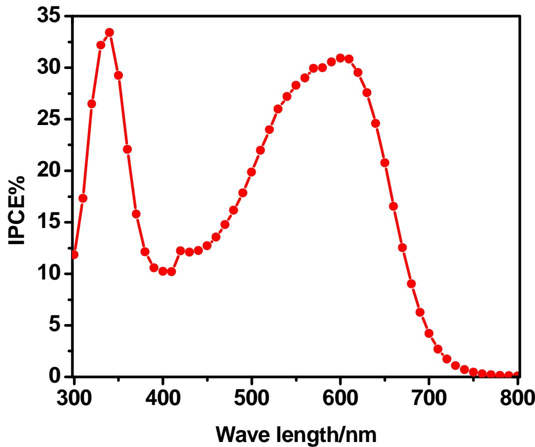
Photocurrent action spectra for ITO/nc-TiO<sub>2</sub>:SH-dye/PVP:CH<sub>3</sub>CN:I<sub>3</sub><sup>-</sup>:EMImI/PEDOT/ITO solid-state PEC.
