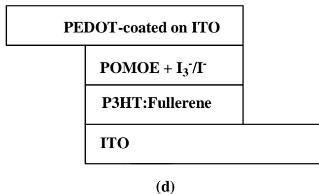
The chemical structure of (a) poly(3-hexylthiophene), P3HT, (b) poly(3,4-ethylenedioxythiophene), PEDOT, and (c) fullerene,  $C_{60}$ , and (d) the basic structure of the solid state PEC.
