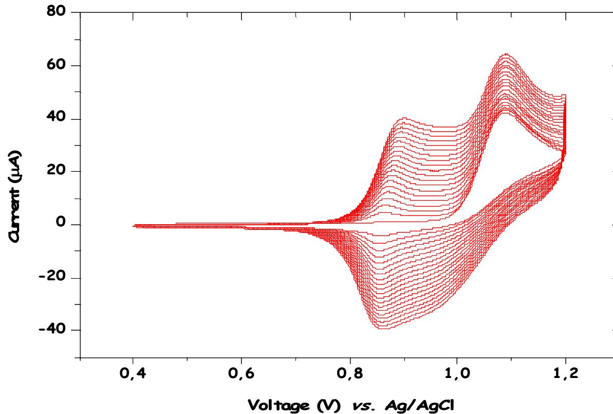
Cyclic voltammogram for the electropolymerization of DHOPT on glassy carbon disk electrode in  $\text{CH}_3\text{CN}$  solution containing 1 mM of the monomers and 0.1 M of TEATFB recorded at a scan rate of 10 mV/s.
