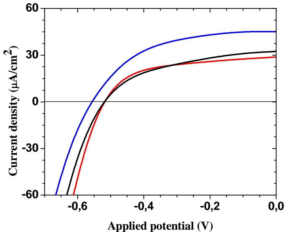
I-V characteristics of the polymer/ $\text{TiO}_2$  based PEC under white light illumination from the backside with light intensity of  $80 \text{ mW}/\text{cm}^2$ :
