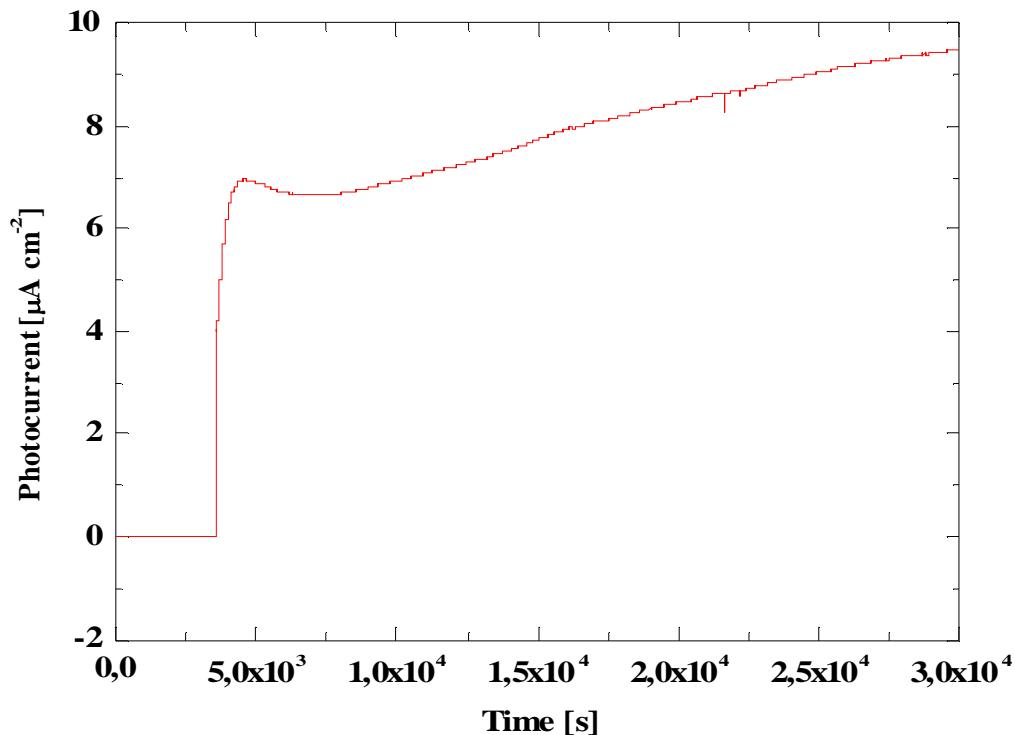
Photocurrent response to continuous illumination with light intensity of 100 mW/cm<sup>2</sup> for P3HT:C60 based solid-state PEC
