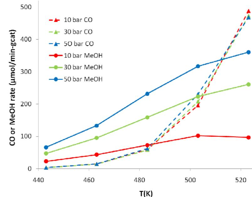
Pressure and Temperature Studies with 200 mg NGM std. Catalyst 20 μm powder
