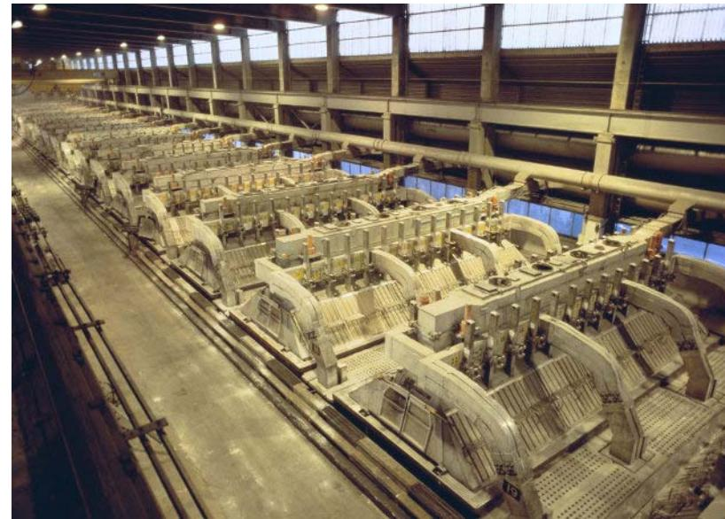
Industrial electrolysis of aluminium oxide
