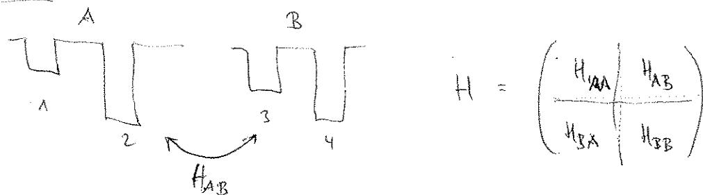
If hopping  $H_{AB}$  comparable to  $t_{12}, t_{34} \Rightarrow$  4 levels with level repulsion
