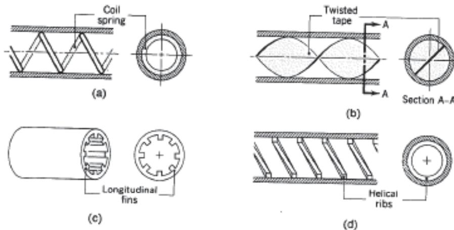
As with normal fluids it is possible to enhance heat transfer in SCF's either for internal tube flow or external flow this can be done with ribs, wire wraps, fins, pins or various other structures.
