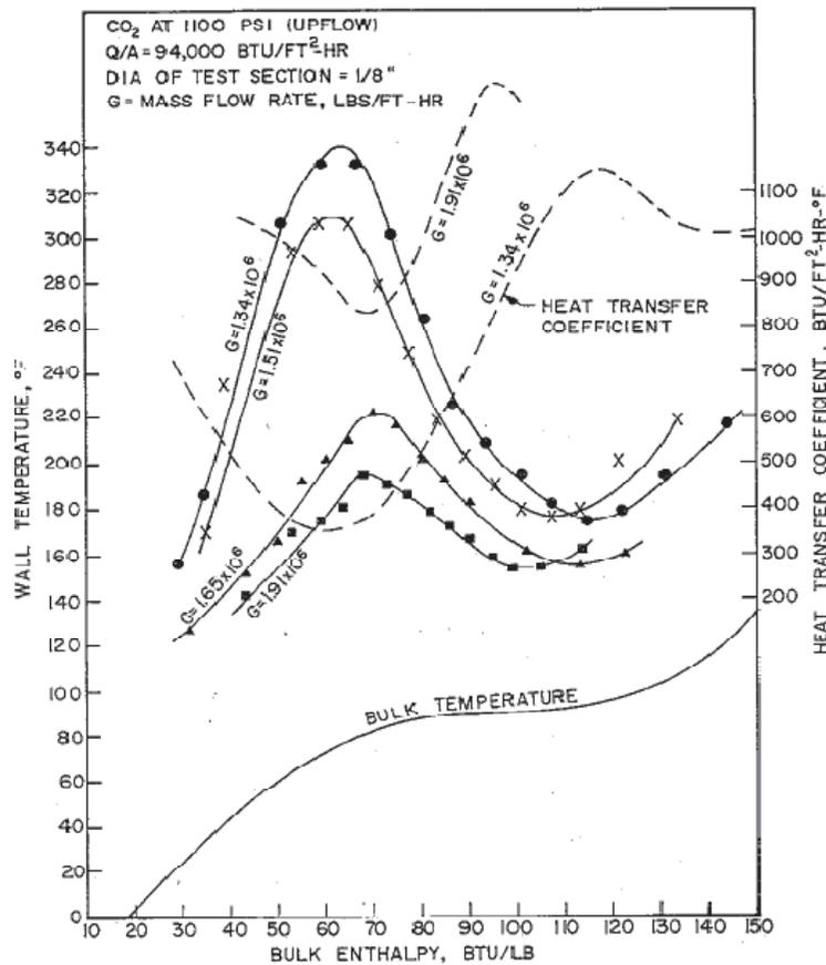
Fig. 3 Variation of the heat transfer coefficient and wall temperature profile for smaller diameter test section
