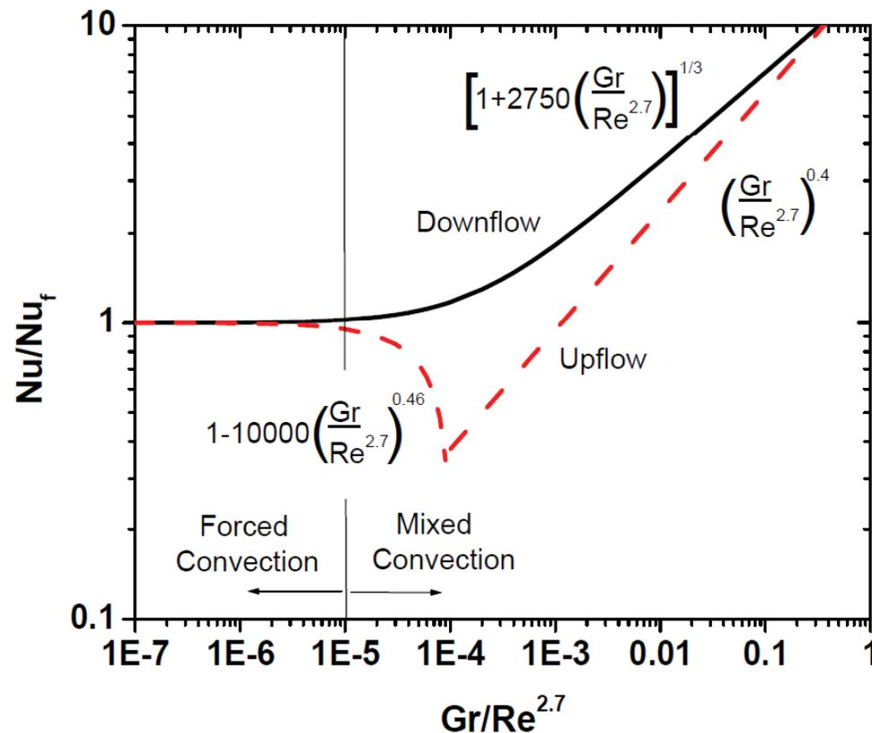
This effect was attributed to a change in the turbulent shear stress due to the influence of buoyancy forces
