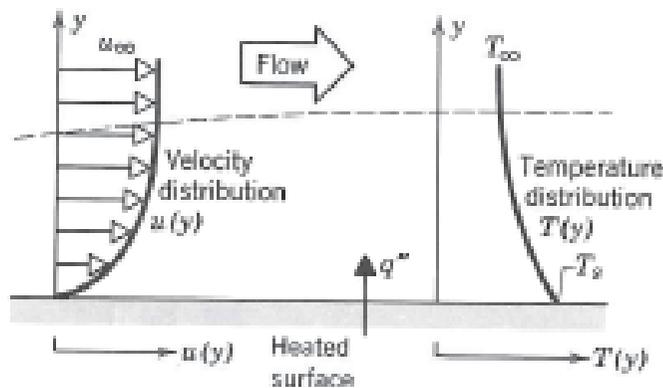
Random molecular motion dominates at  $y$  close to zero. Bulk motion is governed by the boundary layer that develops in the  $x$ -direction. The heat conducted into this layer is swept down stream and eventually transferred to the bulk.
