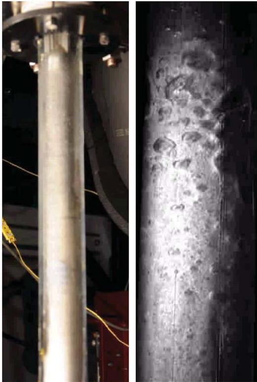
Movies of Simulated TRIGA fuel pin at 3000W atmospheric pressure, inlet temperature 93 C Flow rate ~0.08 kg/s – boiling phenomena
