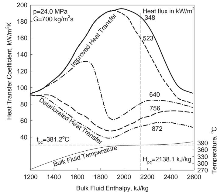
The increase in the buoyancy force in upward flow causes changes in the turbulent boundary layer causing a reduction in the turbulent shear stress (laminar like boundary layer)
