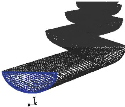
Meshing was performed with hexahedral cells aligned with the predominate flow orientation
