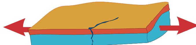
Stress Corrosion (Cracking)
