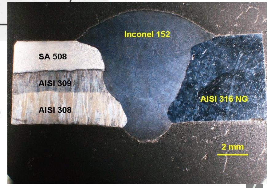
*An example of dissimilar material welding research for main assemblies in RPV*
