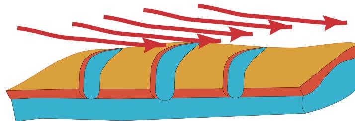
Flow Assisted (Erosion) Corrosion
