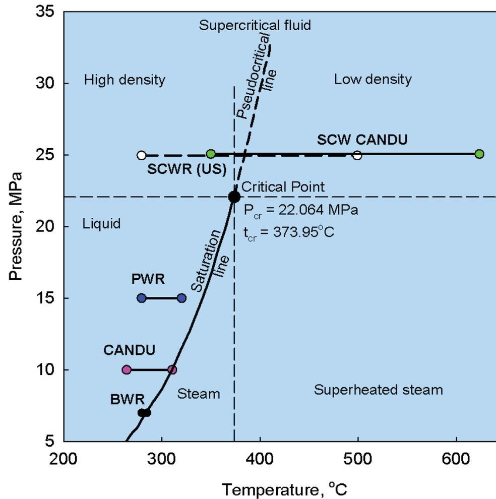
Currently, USA does not develop SCWR concept. However, the shown parameters are typical to other SCWR concepts, for example, HPLWR or Super LWR.
