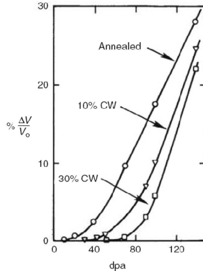
15-15 austenitic SS irradiated at 650°C with 1MeV Cr ions
