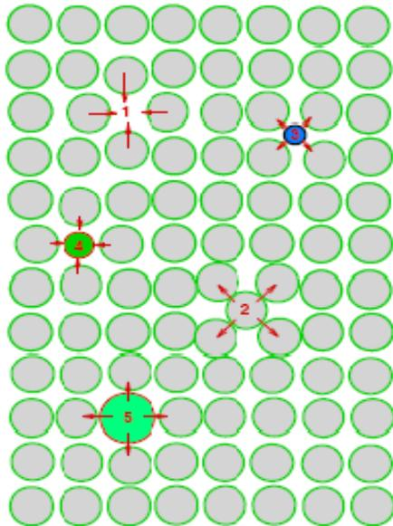
Schematic representation of different point defects in a crystal. (1) vacancy; (2) self-interstitial; (3) interstitial impurity; (4), (5) substitutional impurities. The arrows show the local stresses introduced by the point defects.
