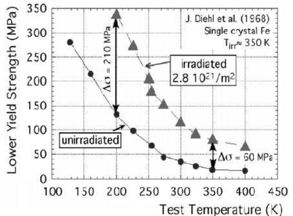
High hardening and loss of uniform elongation occurs for irradiation and test temperatures  $< 0.3 T_M$
