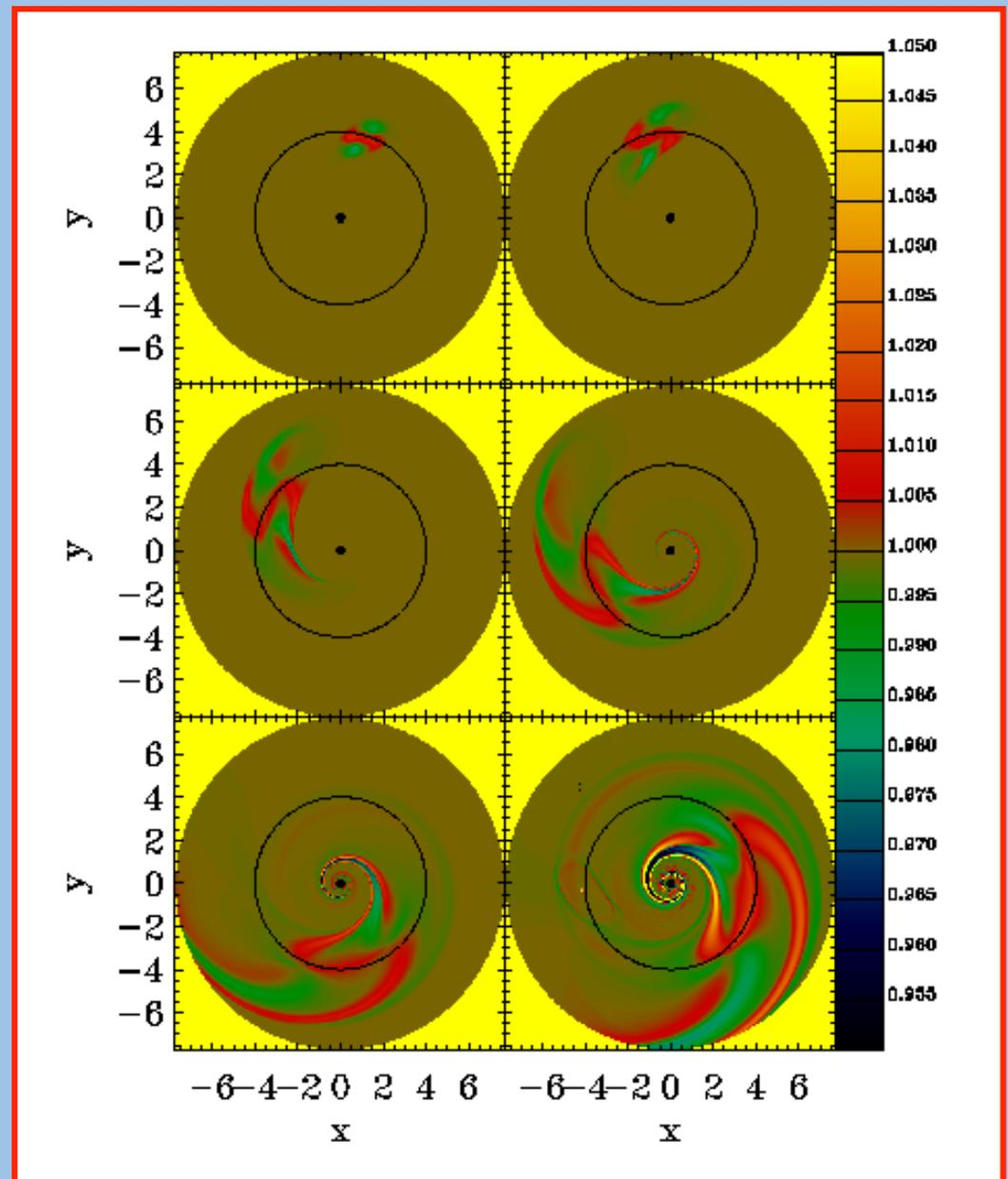
Above: initial vorticity perturbation; left: density (6 different times) Note the emergence of the wave (2nd panel) and the triggering of the global spiral mode.
