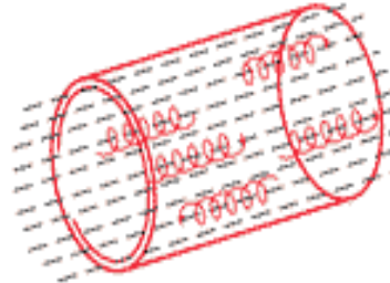
Motion of charged particles with magnetic field.
