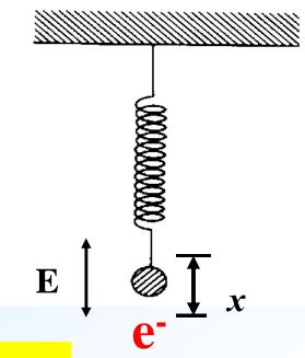
$$p = -ex = \frac{e^2}{m(\omega_0^2 - \omega^2 + i\omega\gamma)} \cdot E_0 e^{i\omega t}$$
