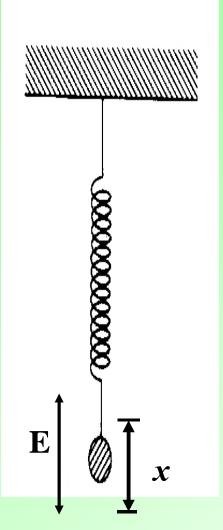
If the force exercised by the electric field of the wave becomes comparable with the Coulomb's force between the electron and the nucleus, the oscillator is perturbed (anharmonic oscillator) and, at the lower level of the perturbation, we can write:
