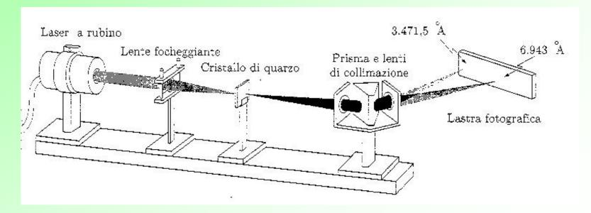
To describe the phenomenon, it is necessary to observe that in many crystal materials the nonlinear polarization depends on the **direction of propagation**, on the polarization of the electric field and on the orientation of the optical axis of the crystal. Since in such materials the vectors  $\mathbf{P}$  and  $\mathbf{E}$  are not necessarily parallel, the coefficient  $\chi$  is a tensor. The second order polarization can be written as
