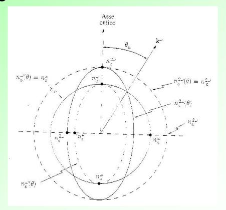
The angle  $\vartheta_n$  is determined by the intersection between the sphere (shown as a circle in the figure) which corresponds to the index surface of the ordinary beam to  $\omega$  with the index ellipsoid of the extraordinary beam. The angle  $\vartheta_n$ , for negative uniaxial crystals (that is for crystals for which  $n_s^{(2\omega)} < n_0^{(\omega)}$  is given by
