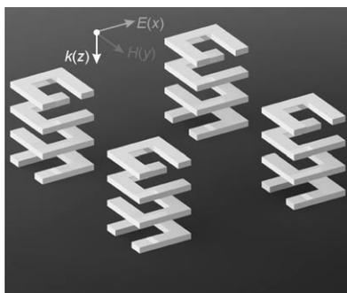
**Figure 15.** Geometry of a four-layer twisted split-ring metamaterial. The size of each split ring is  $400 \times 400 \text{ nm}^2$ . The arm width is 100 nm and the gold thickness is 60 nm. The vertical spacing between the adjacent split rings is 60 nm. The normally incident light is polarized along the gap-bearing side of the top split ring. Reprinted from Ref. [42], with permission from the Optical Society of America.
