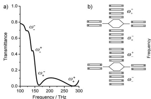
**Figure 14.** Simulated transmittance spectrum for four coupled nanowires. The size of the individual nanowires is  $500 \times 150 \times 20 \text{ nm}^3$ . The vertical spacing between nanowires is 80 nm. The light is incident along the stacking direction, with a linear polarization along the longer axis of the nanowires. b) Schematic illustration of the resonance diagram depicting the hybridization of the modes for the stacked nanowire structure. Reprinted from Ref. [40].
