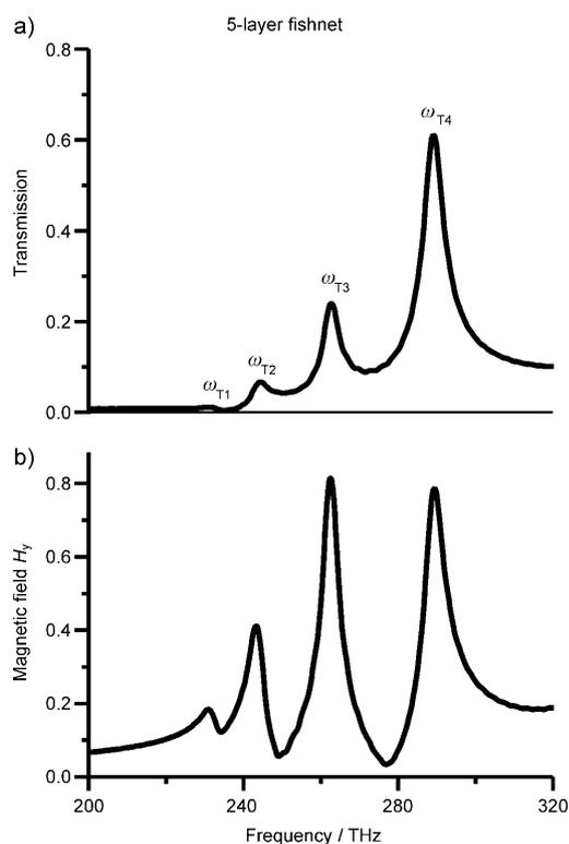
**Figure 19.** a) Simulated transmission spectrum and b) detected  $H_y$  intensities for the five-layer fishnet metamaterial. The  $H_y$  probe is positioned inside the gap between the top two gold wires. Reprinted from Ref. [42], with permission from the Optical Society of America.
