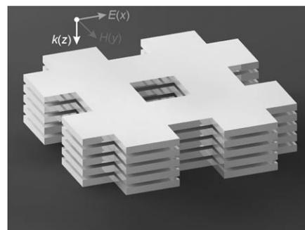
**Figure 18.** Geometry of a five-layer fishnet metamaterial. The width of each wire is 350 nm. The thickness of the gold is 40 nm and the vertical spacing between wires is 20 nm. The normally incident light is polarized along the  $x$  direction. Reprinted from Ref. [42], with permission from Optical Society of America.
