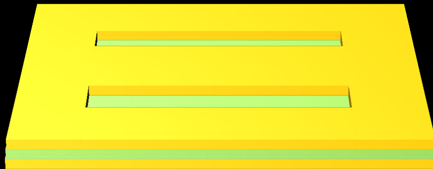
Alternating Gold slits removed by FIB
